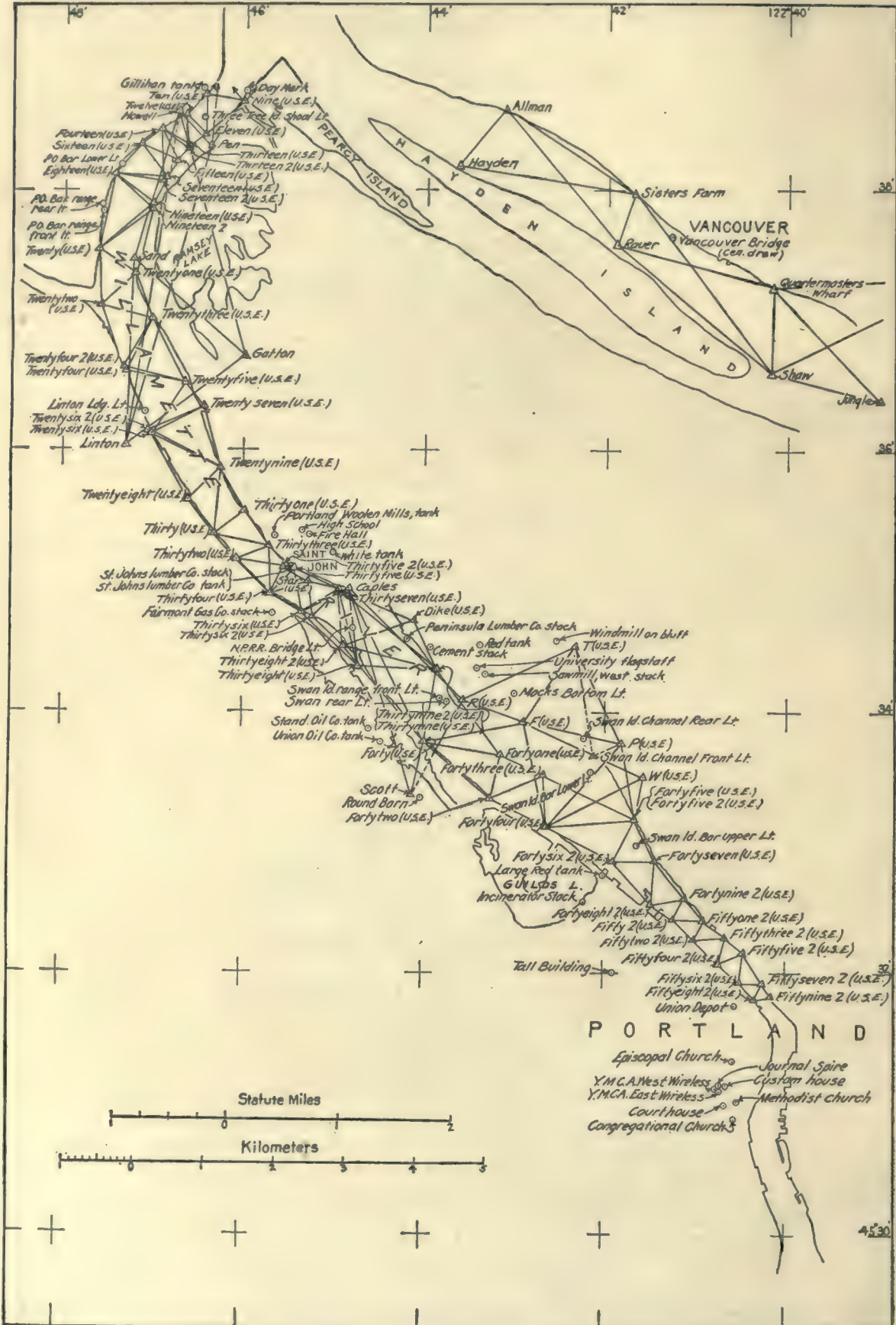
FIG. 19.—TRIANGULATION, MOUTH OF THE WILLAMETTE RIVER TO PORTLAND.
